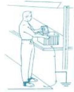
Part of the path-to-ground is the perspiration in the person's shoes. Foot grounder conductive tabs or ribbons should be placed inside the shoe under the foot with the excess length tucked into the shoe. Thanks to the perspiration in the shoe, direct contact with the skin is normally not necessary.
