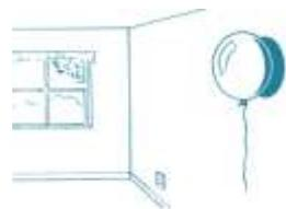
isolated conductors can be conductive traces or components loaded on a PC board that is not in contact with the ESD worksurface. Reduction of charges on insulators does occur naturally by a process called neutralization. Ions are charged particles that are normally present in the air, & as opposite charges attract, charges will be neutralized over time. A common example is a balloon rubbed against clothing & "stuck" on a wall by static charge.
